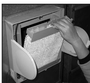
9. Place the drip tray on top of the pad. Reinstall the evaporator pad and drip tray.
