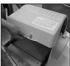
4. Tilt and lift the cover off the frame.
