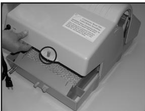
4. Remove the cover by turning the thumb screw (circled) counterclockwise (↺). Tilt and lift the cover off the frame.
