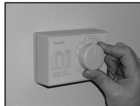
**15.** Test operation. Check for water leaks. Be sure the humidistat is operating properly. Installation is now complete.
