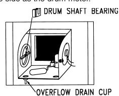
**2.** On the inside of the cabinet where the bypass tube will connect, snap the drum shaft bearing in place with the "U" shape of the bearing pointing up.
