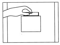
1. After determining the best location for the humidifier, draw a level line on the plenum and tape the template in position. Trace around the template, then remove template and connect any blank spaces where the tape was removed. Now carefully cut the rectangular opening. Insert cabinet in opening and make sure it is level. Mark the location of the five mounting holes. Remove cabinet and drill five 7/64" mounting holes. Replace the cabinet and secure with self tapping screws
