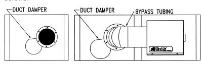
**3.** Install the 6" collar on the other plenum and connect a 6" bypass tube from the collar to the unit with sheet metal screws. Seal connections with duct tape. If the furnace has air conditioning, install the duct damper for summer season shutoff.
