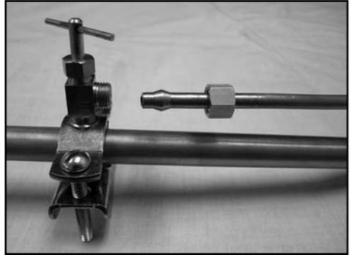
4. Route the tubing to the humidifier float valve, keeping the tubing away from sharp edges.
