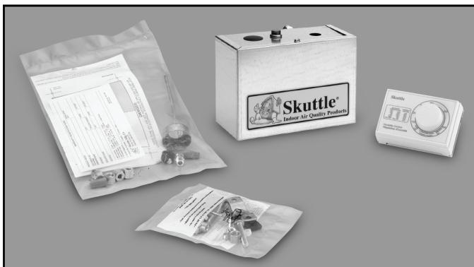
**Installation Package** includes a Skuttle manual humidistat, self-piercing saddle valve, mounting template, mounting hardware, observation window and installation instructions.
